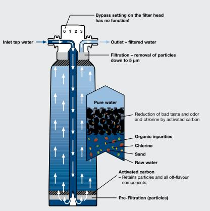
Cross-Section of a BWT besttaste filter cartridge
